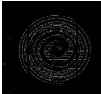
Fig. 3: Swirl defect after application of the Canny edge detector
