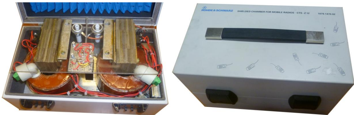
Fig. 2: Design and realization of the AC Power Supply 2x6 kV.
