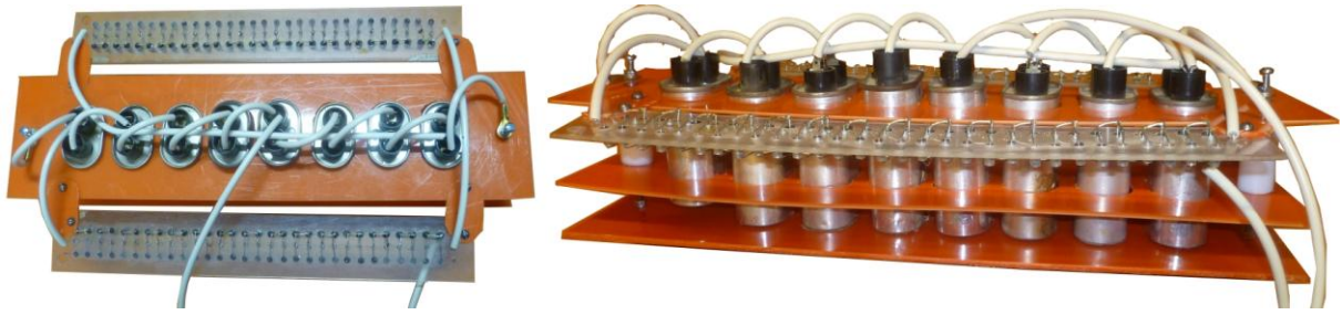
Fig. 3: The high voltage rectifier with multiplier and capacitor filter
