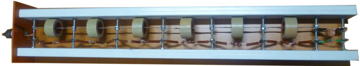
Fig. 4: The high voltage RC divider
