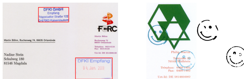
Figure 2: On the left, stamps extracted by the algorithm are marked by red bounding boxes. On the right, correctly segmented overlapped stamps are shown.
