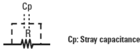
Fig 2: Real-world high value resistor
